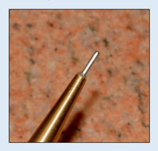
Insert into the Core. Use gentle, even pressure to insert the pin into the core. Make sure the pin is inserted straight, avoiding distortion or early wear of the hole.
