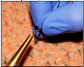
Place one High-Flow Cone Pin (P/N H076110608) into the Pin Driver Tool.
